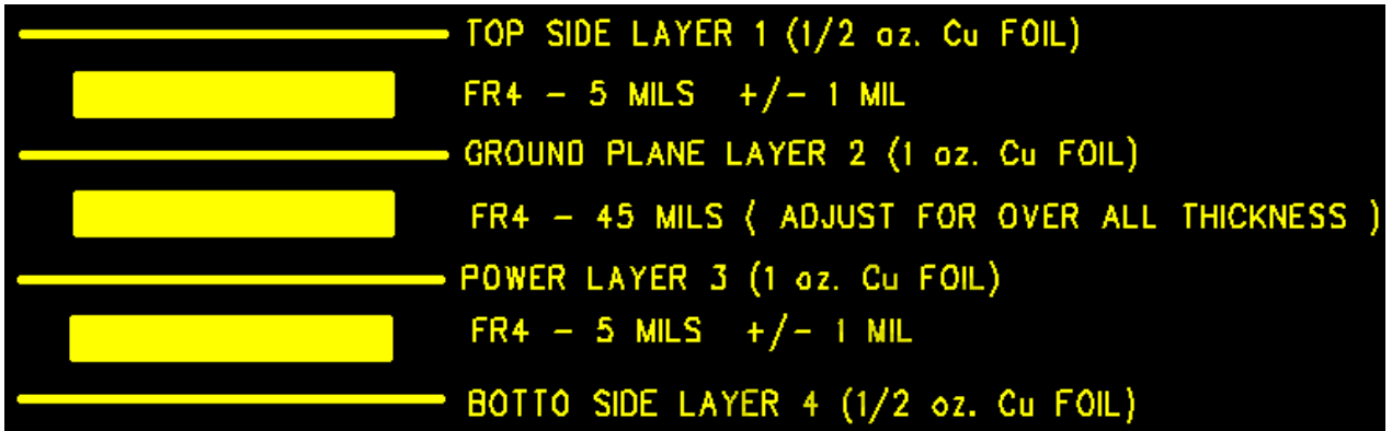
Figure 4 - Board Stack-Up
