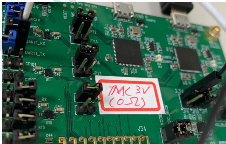
Figure 27 - UART Console Pin of Interface Board
