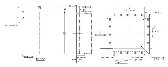
Table 4.3-1 ATM2231/ATM2231U 56-Pin 7x7 mm QFN Dimensions
