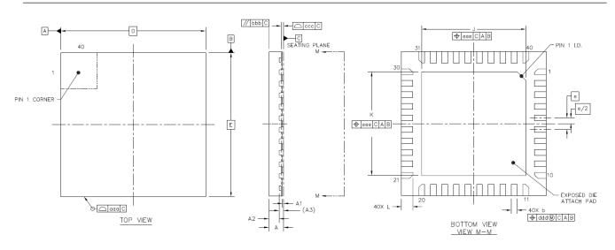
Table 4.1-1 ATM2201 40-Pin 5x5 mm QFN Dimensions
