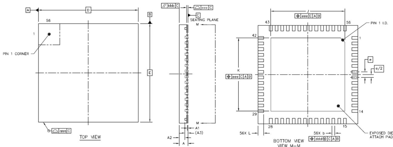
Table 4.3-1 ATM2231/ATM2231U 56-Pin 7x7 mm QFN Dimensions
