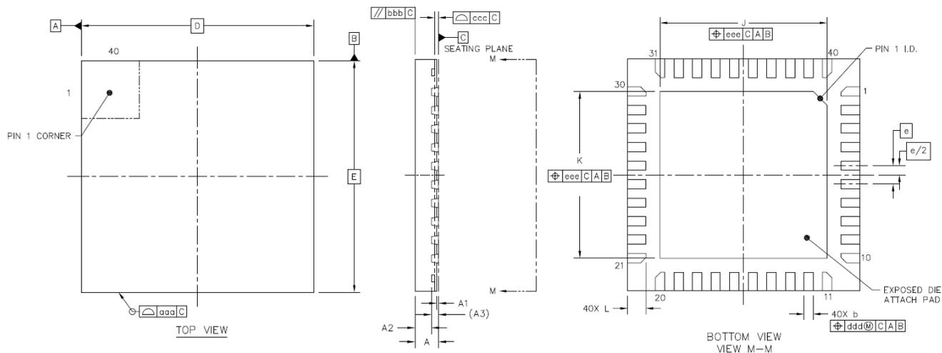
Table 4.1-1 ATM2201 40-Pin 5x5 mm QFN Dimensions
