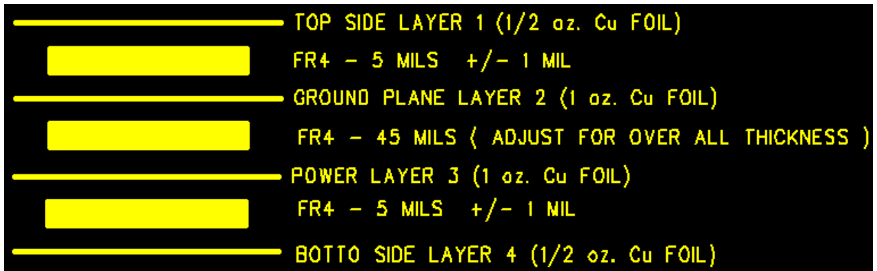
Figure 5 - Board Stack-Up
