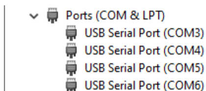
Figure 6-5 COM Port Setup in Device Manager
