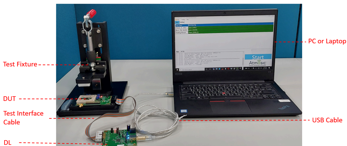
Figure 3-2 Connection Setup Between PC, DL, and DUT
