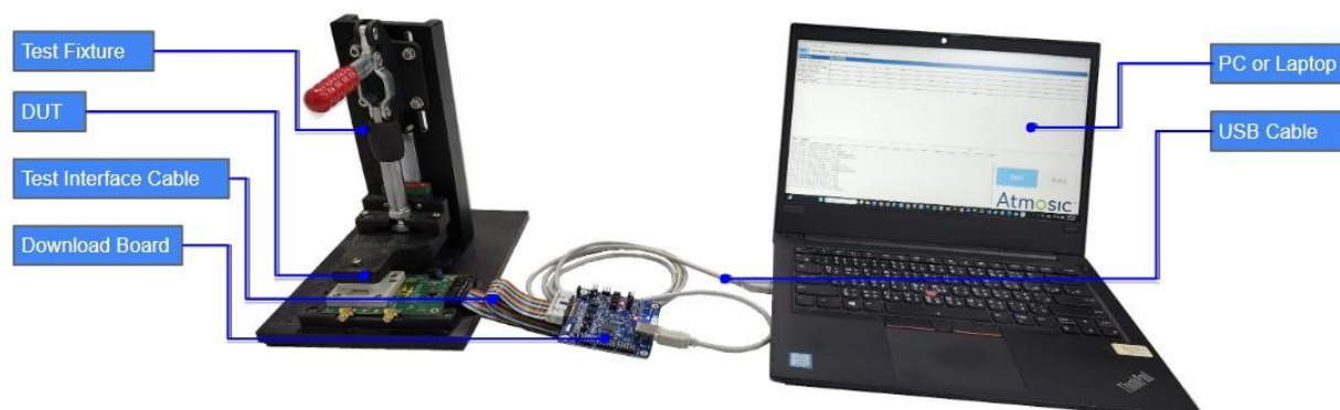
Figure 3-2 Connection Setup Between PC, Production Download Board (DL), and DUT
