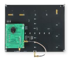
Figure 4 - Locator Antenna Array (Bottom Side)
