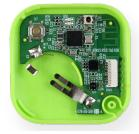
The Tag is powered by a coin cell battery (included) and transmits its beacon from the 2.4 GHz Bluetooth antenna on the Tag.
