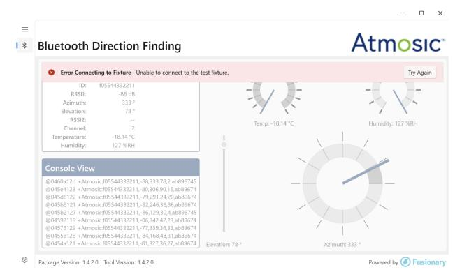
Figure 12 - USB Cable Connected But No Connection Recognized
