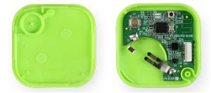
Figure 1 - ATM3325 Tag Reference Design
