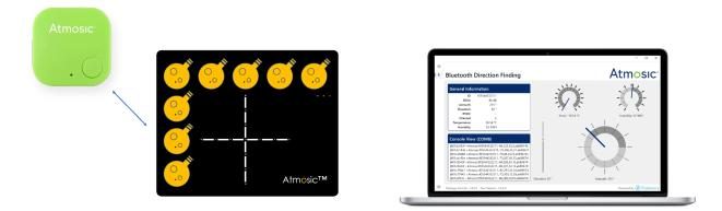
Figure 9 - GUI Display if Tag is Located on the left of the Locator
