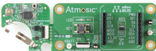
Figure 2 - ATM3325 Tag Reference Board with Sensor Extension
