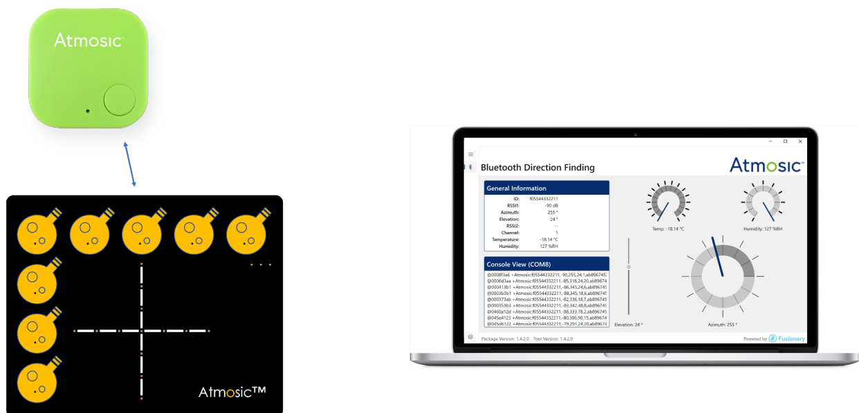
Figure 10 - GUI Display if Tag is Above the Locator
