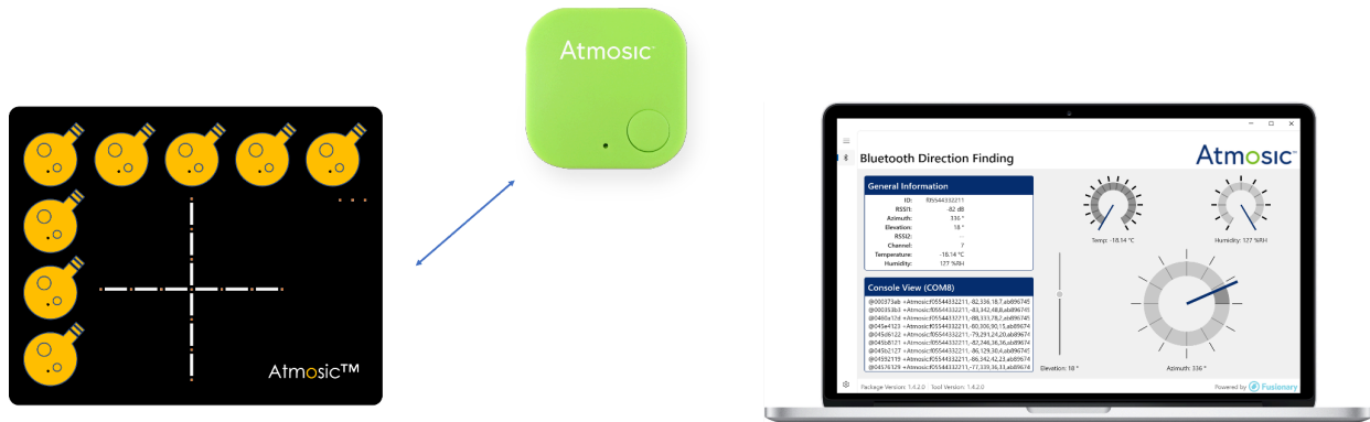
Figure 11 - GUI Display if Tag is Located on the Right of the Locator
