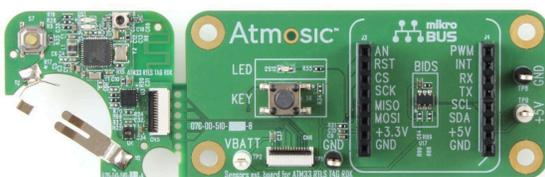
Figure 2 - ATM3325 Tag Reference Board with Sensor Extension
