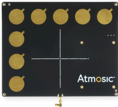
Figure 3 - Locator Antenna Array (Top Side)
