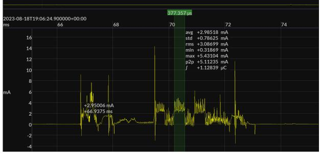
Figure 6 - Transmit Current Profile
