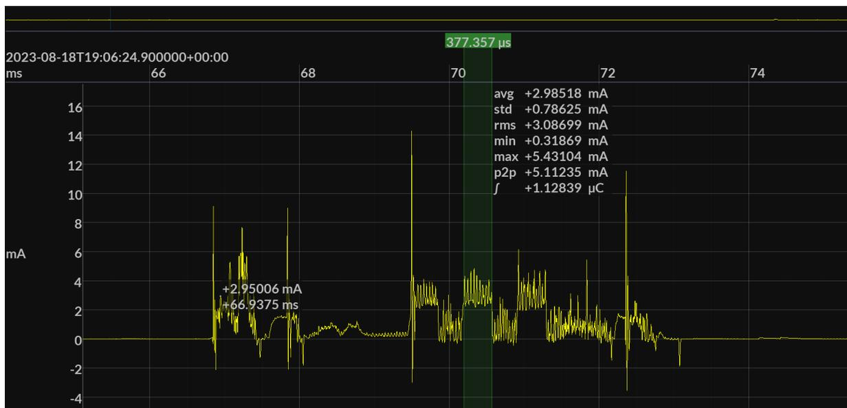
Figure 6 - Transmit Current Profile
