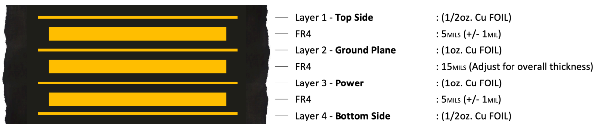
Figure 13 - 4-Layer Stack-up for Thinner PCB
