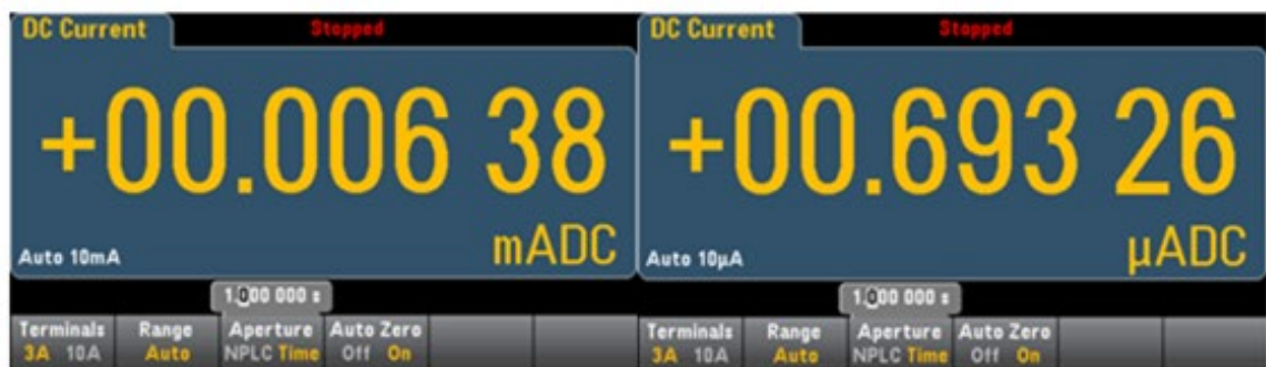
Figure 7 - Average Power Measurement with Multimeter
