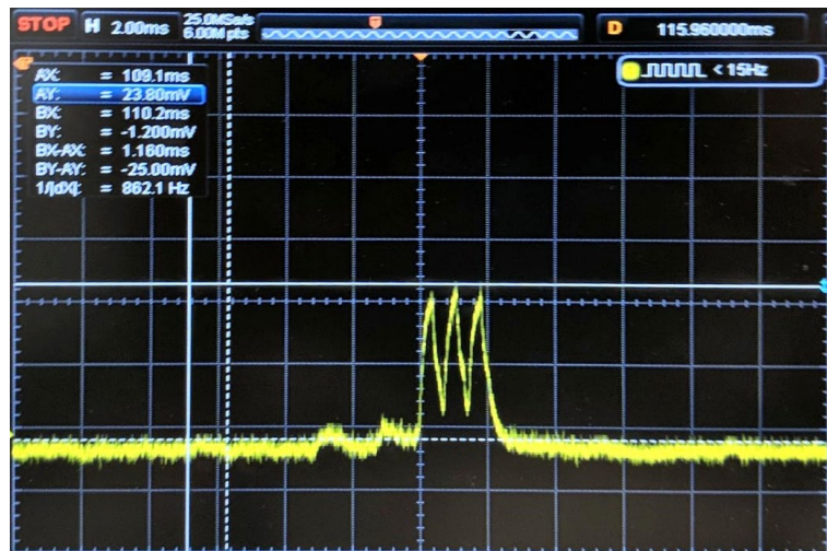
Figure 8 - Approximate Power Profile Measurement
