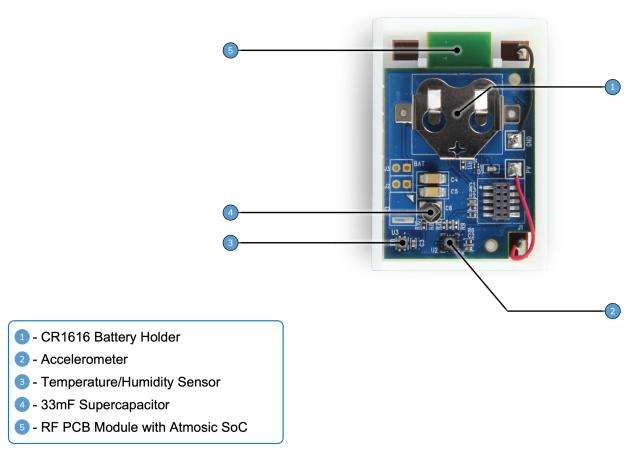
Figure 2 - Inside of the PV Beacon
