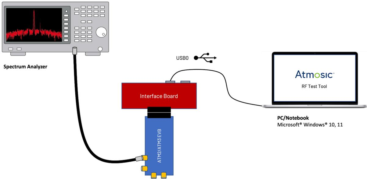
Figure 13 - ATM2/ATM3 EVK Tx Test Environment Setting
