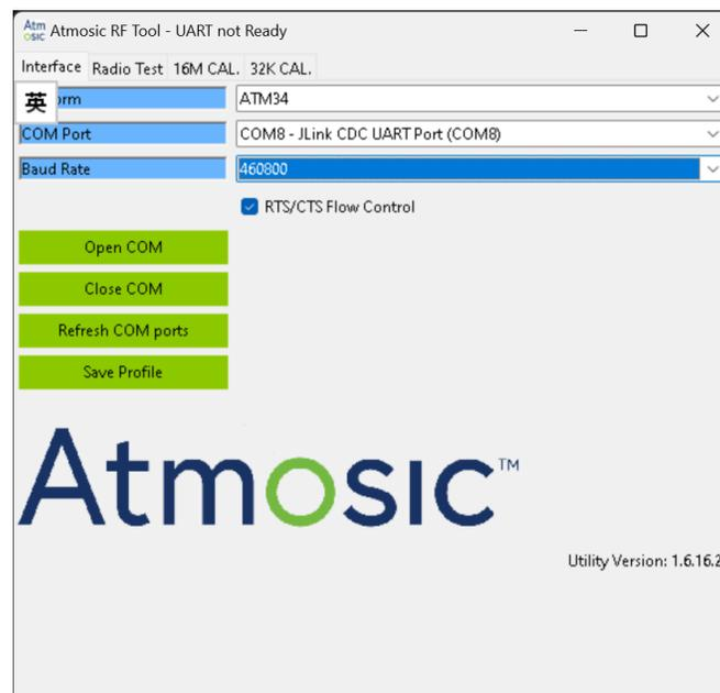
*Figure 10 - RF Test Tool Interface Setting*
