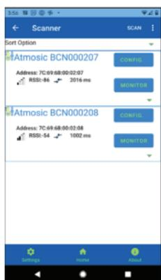
The sensor data displayed includes the Received Signal Strength from the sensor (RSSI), Temperature, Humidity, and accelerometer data:
