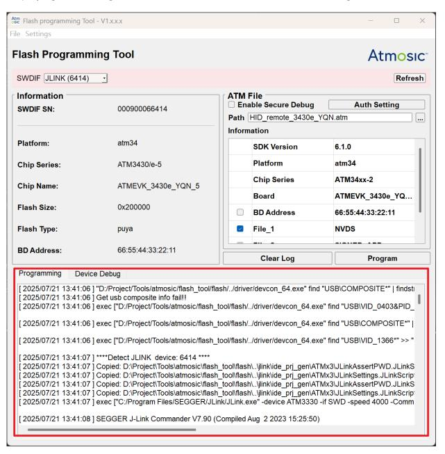
Figure 3-6 Programming Log in Main GUI
