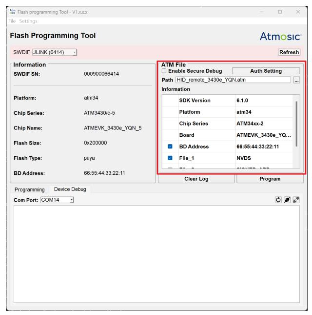
Figure 3-3 ATM File in Main GUI
