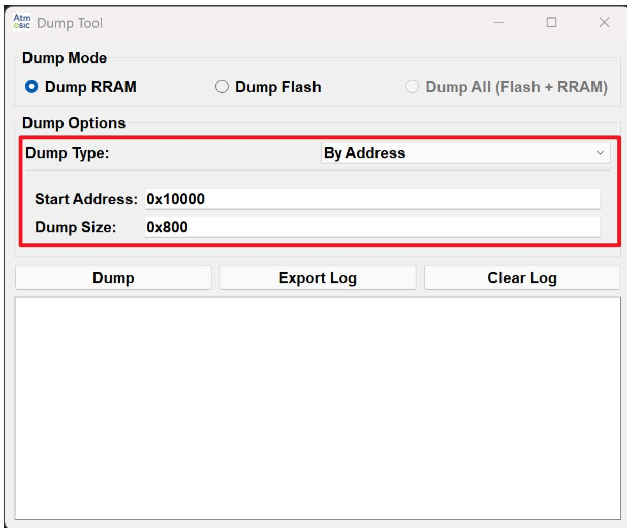
Figure 7-4      *Dump Type (By Address)*
