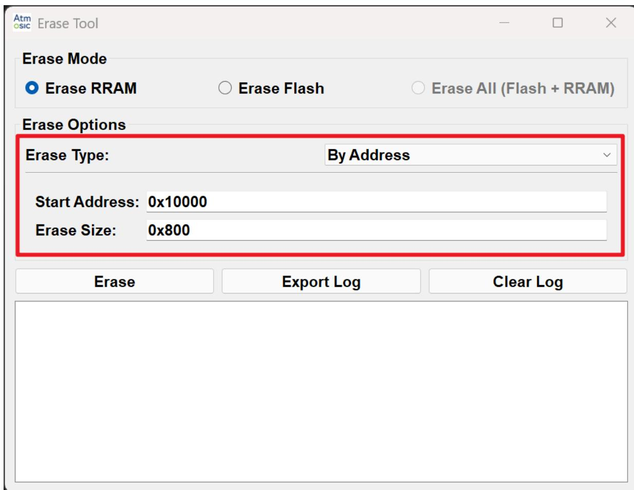
Figure 8-4      *Erase Type (By Address)*
