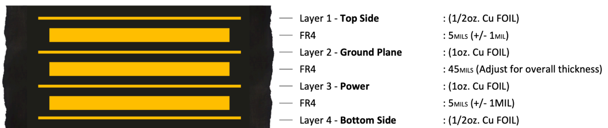
Figure 6-4 - Board Stack-Up
