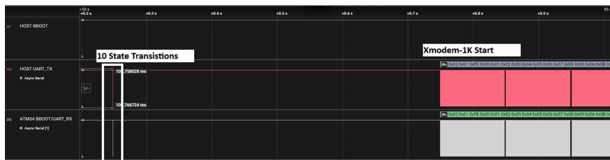
Figure 3-2 - Timing Diagram for Option #1 - Separate BBOOT (P25) and UART1 RX (P25)
